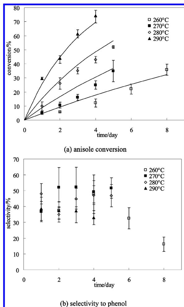
Figure 3. Temporal variation of anisole conversion and selectivity to phenol at different temperatures.
