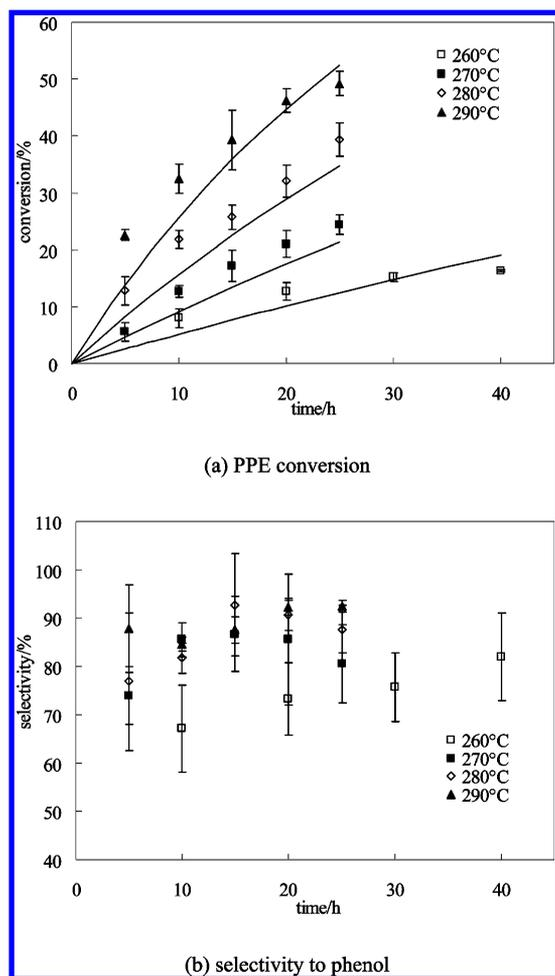
Figure 6. Temporal variation of PPE conversion and selectivity to phenol at different temperatures.
