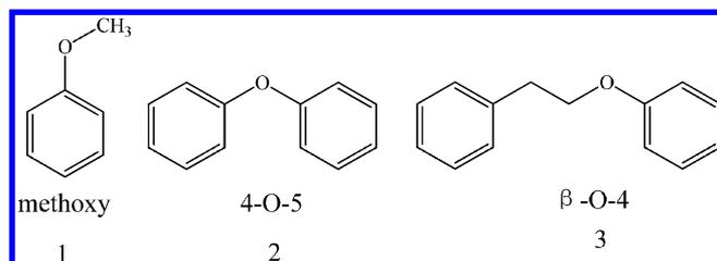
**Figure 1.** Structure of lignin model compounds in this study: (1) anisole, (2) diphenyl ether, (3) phenethyl phenyl ether.
