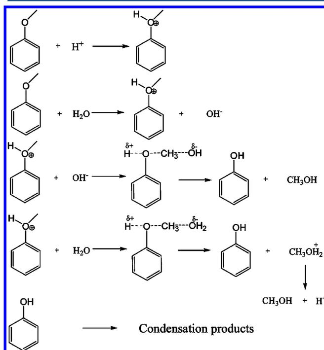
Figure 4. Proposed reaction mechanism for decomposition of anisole.
