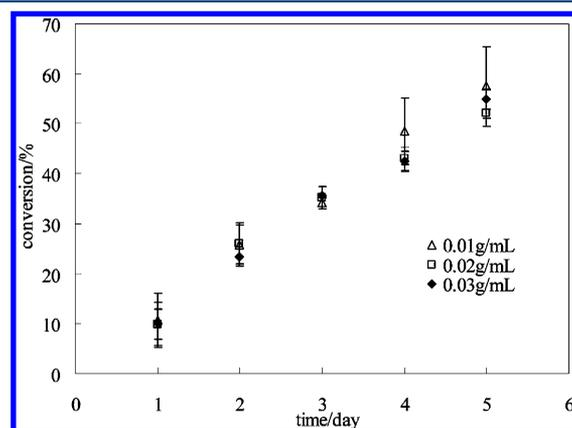
**Figure 2.** Temporal variation of anisole conversion at different initial concentrations.
